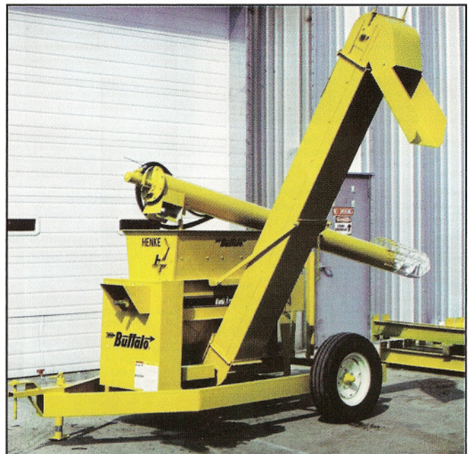
Elevator discharge on a trailer-mounted mill.
