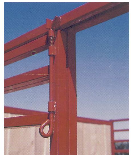
Overhead latch locks sliding door open or closed.
